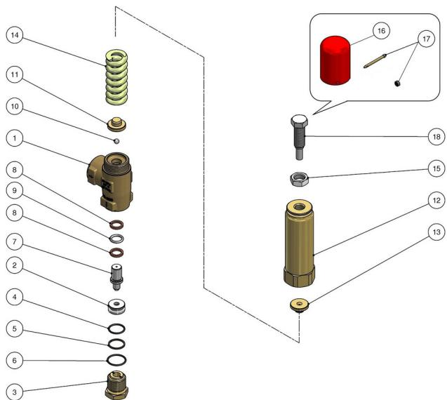
60.5230.00 VS500/310 safety valv. 1/2F Bsp bypass:3/4F
